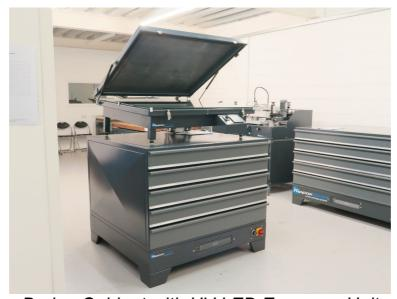
Drying Cabinet with UV LED Exposure Unit
